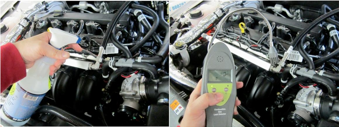
15. If there is a leak, add an additional ¼ turn to the low pressure hose connection. Perform another leak test. If leak persists, notify your supervisor for further instructions.
