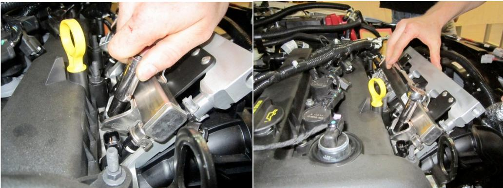
7. Tighten the fuel rail brackets using an Allen wrench.
