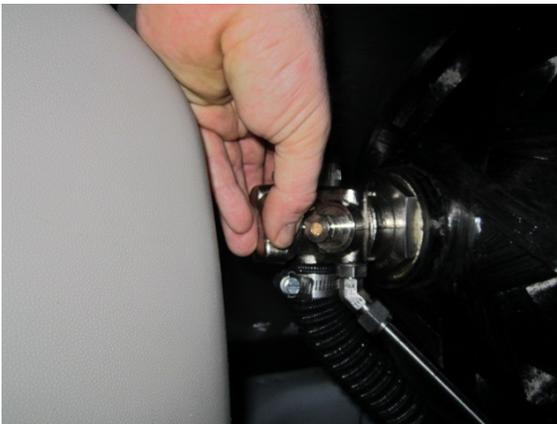
3. If vehicle is **operational** (does not apply to Bi-Fuel systems), depressurize the system by running the vehicle on CNG until the vehicle stalls. As an extra safety precaution, also crack the low pressure hose one half turn at a time to ensure all pressure has been vented. If the vehicle is **not**
