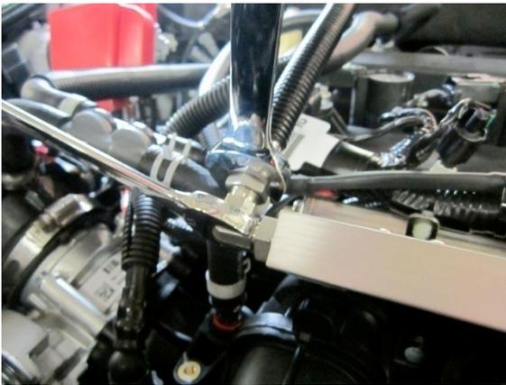
15. Connect the vehicle battery, open the valve(s) completely and back  $\frac{1}{4}$  turn, and re-pressurize the system using 3 key on/off cycles.
