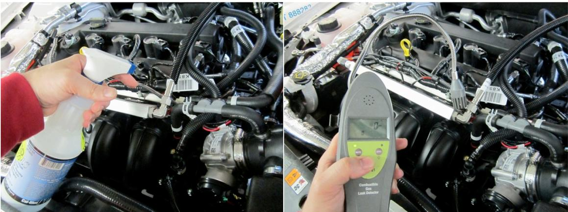
17. If there is a leak, add an additional  $\frac{1}{4}$  turn to the low pressure hose connection. Leaks originating from injector connection points indicate a
