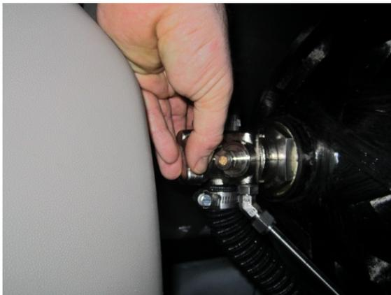
3. If vehicle is **operational** (does not apply to Bi-Fuel systems), depressurize the system by running the vehicle on CNG until the vehicle stalls. As an
