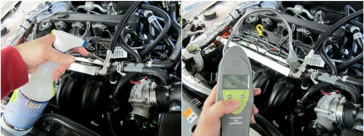
12. If there is a leak, add an additional  $\frac{1}{4}$  turn to the low pressure hose and or transducer. Perform another leak test. If leak persists, notify your supervisor for further instructions.
