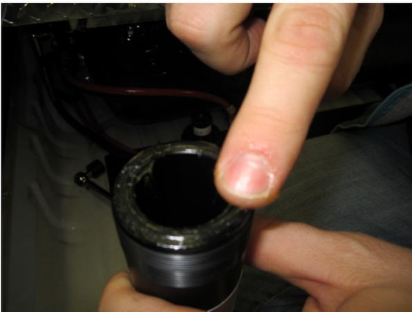
8. Install seal (Small O-ring included in filter packaging.) to the top of the filter. Apply Parker lube and install new filter. Filter will snap into place when installed into its corresponding hole located inside top filter housing.
