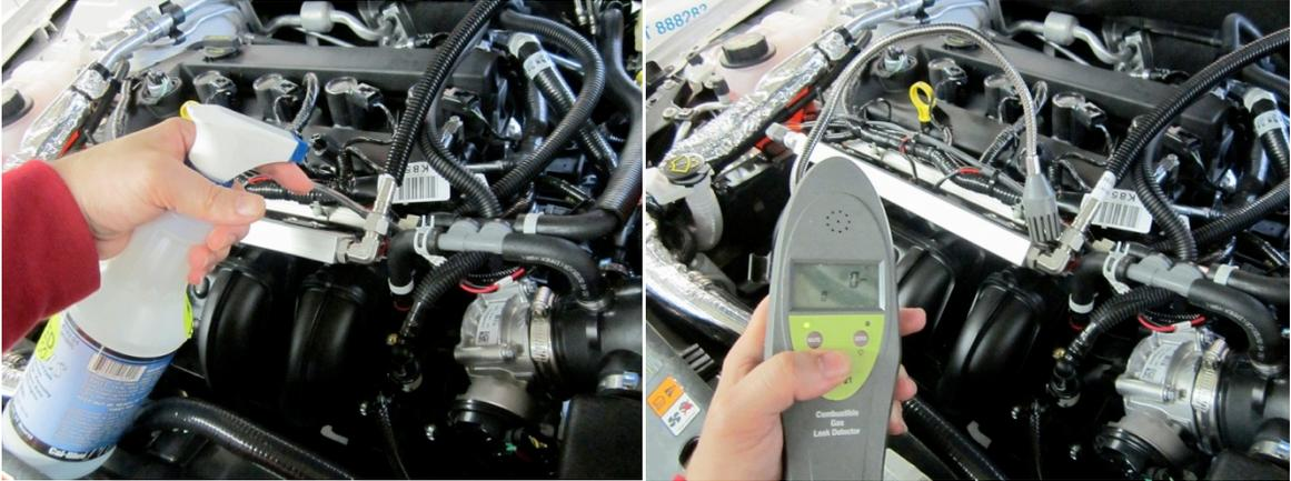
11. If there is a leak, add an additional  $\frac{1}{4}$  turn to the low pressure hose connection. Perform another leak test. If leak persists, notify your supervisor for further instructions.
