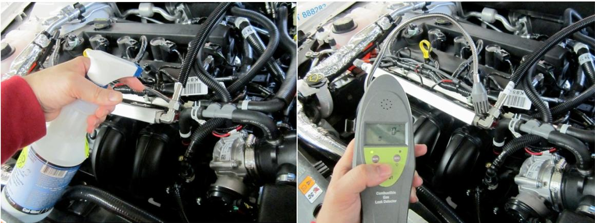
14. If there is a leak, add an additional ¼ turn to the low pressure hose connection or transducer connection. Perform another leak test. If leak persists, notify your supervisor for further instructions
