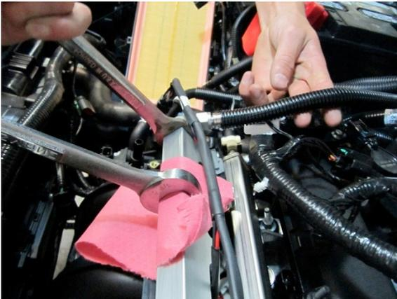
10. Connect harness plug to transducer and connect the low pressure hose. To tighten the low pressure hose, first hand tighten as much as possible, then make
