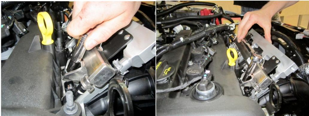
12. Tighten the fuel rail brackets using an Allen wrench.
