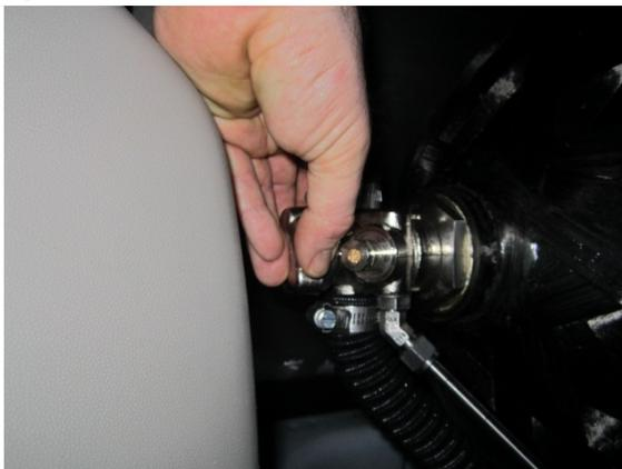
3. If vehicle is **operational** (does not apply to Bi-Fuel systems), depressurize the system by running the vehicle on CNG until the vehicle stalls. As an extra safety precaution, also crack the low pressure hose one half turn at a time to ensure all pressure has been vented. If the vehicle is **not operational**, crack and loosen the low pressure hose on the fuel rail side one half turn at a time until all pressure has been vented. Completely disconnect the low pressure hose.
