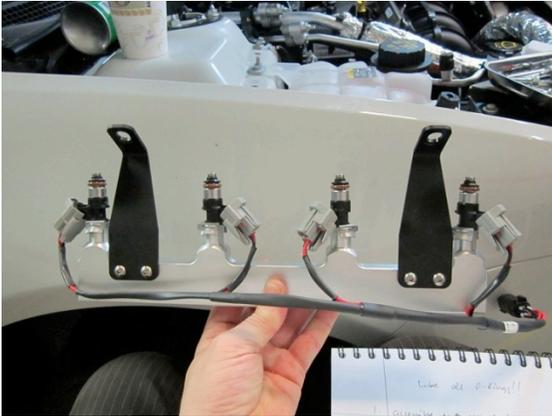
5. Plug all injector connections, then carefully nudge fuel rail evenly from side to side and ease it into place to avoid o-ring damage.
