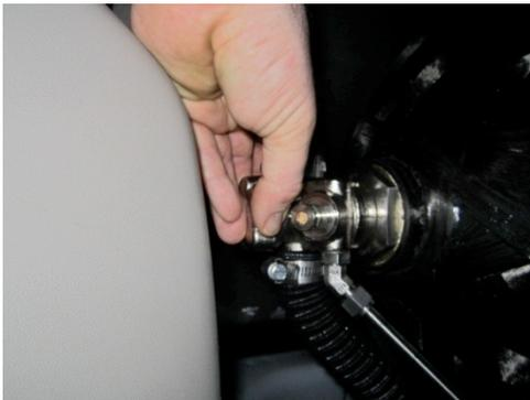
3. If vehicle is **operational** (does not apply to Bi-Fuel systems), depressurize the system by running the vehicle on CNG until the vehicle stalls. As an extra safety precaution, also crack the low pressure hose one half turn at a
