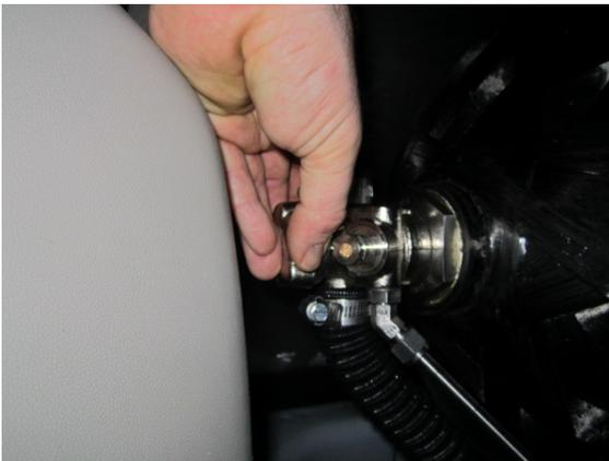
3. Clamp the OEM coolant hoses to restrict coolant flow. Work on one hose end at a time.
