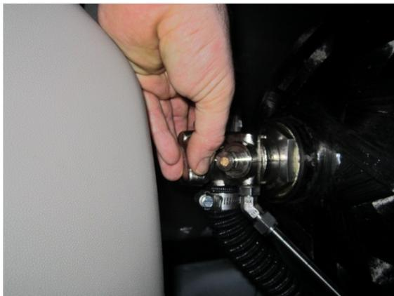
3. If vehicle is **operational** (does not apply to Bi-Fuel systems), depressurize the system by running the vehicle on CNG until the vehicle stalls. As an extra safety precaution, also crack the low pressure hose one half turn at a time to ensure all pressure has been vented. If the vehicle is **not operational**, crack and loosen the low pressure hose on the fuel rail side one half turn at a time until all pressure has been vented.
