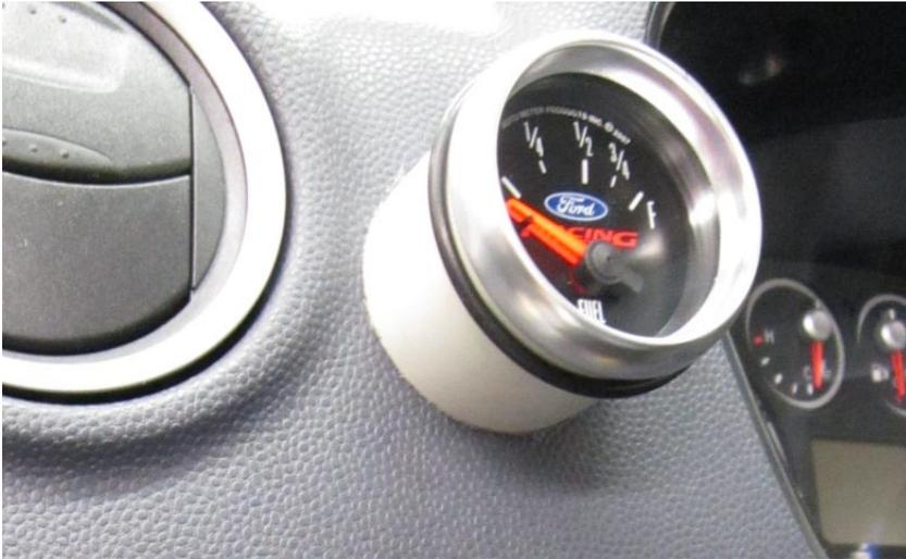
4. Replace fuel gauge. Ensure harness connections to fuel gauge are correct.
