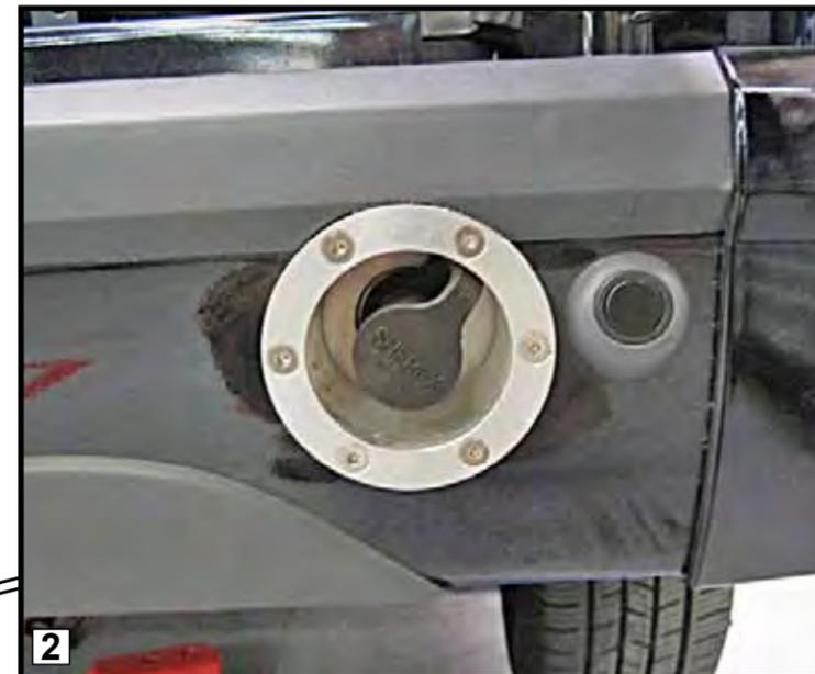
Installed Fuel fill With backup sensor. Torque six hex bolts to 35-40in lb.
