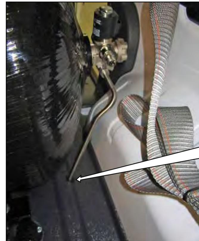
To prevent vibration open up the hole in the frame to 3/4".
