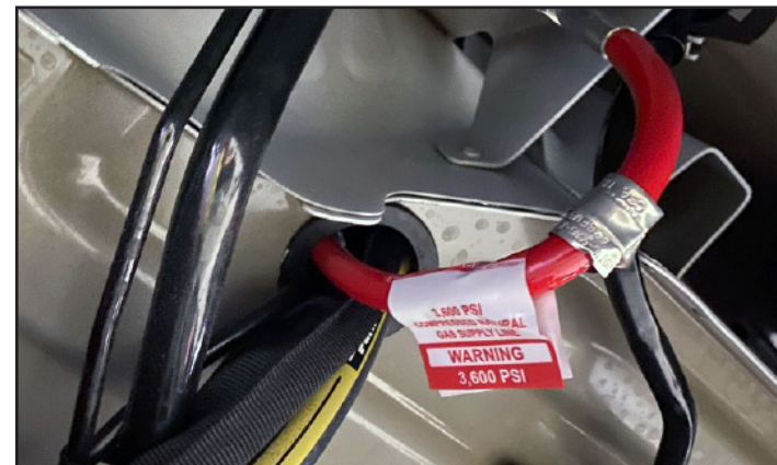
All high pressure hoses must be labeled with a high pressure sticker.
